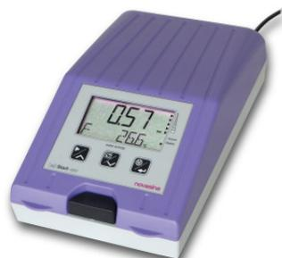
**Portable low cost precision instrument for water activity measurement ( $a_w$ ) in foodstuff and powder products**
