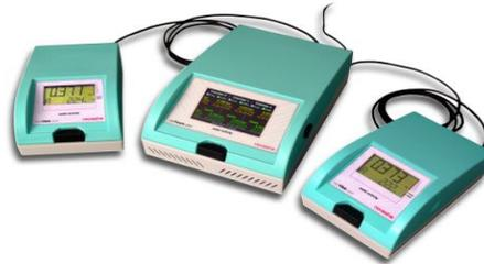
The flexible **LabTouch-aw** system can be extended by max. 2 additional external **LabClick-aw** chambers. This offers a higher measurement capacity running 2 or 3 chambers contemporaneously. The calibration and system management is made by the **LabTouch-aw** "ADVANCED". The external chambers can be put in a climatic chamber if required.
