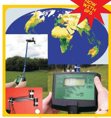
The meter features automatic datalogging and a solar radiation integration function as MJ/day solar energy.
